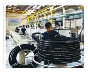
High-Pressure Hydraulic Hoses which are primarily used for heavy industry and mining industry. Through jointly partnership between the Company and Semperit Technische Produkte, this company has a total capacity of 42.5 million metres per annum from the production in Thailand and the PRC and has a distribution networks around the world.
